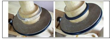
The O-rings are simply inserted onto the thicker portion of the spindle, about halfway up from the bottom. They will stay in place when you are inserting and removing cones. If they shift in position, simply adjust them. The clear o-ring is used with our cones.
