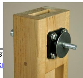
1 - The first step is to install the large 2" diameter steel washer onto the shaft. Press against the back of the shaft to keep it from moving out of position when installing all of these parts. Put the smooth part of washer against the bearing.
