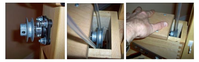
Attach the metal pulley to the end of the HDSS shaft as pictured above. It is important that the groove in this pulley is directly above the pulley in the motor housing. If you must reverse this pulley in order to get the grooves to align properly, then do that. Tighten the set screw with the Allen wrench. <u>Make sure</u> the pulley is positioned such that the set screw makes contact with the FLAT portion of the shaft.
