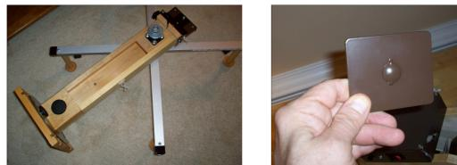
You will pre-position the HDSS upside down on its side on the floor so that you can easily install the motor housing while the HDSS is laying face down. While in this position, it is easier to install the heavy motor housing onto the I-beam.
