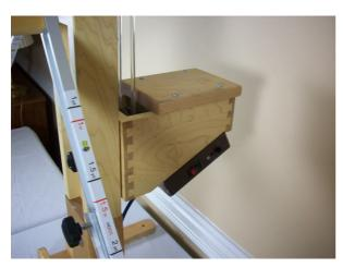
The switch closest to the front (toward the I-Beam) is the **On/Off switch** (it has the International symbols for on (a vertical line) and off (a circle)). <u>This switch must</u> <u>be on in order for the unit to run</u>. Note: these pictures are of a prototype unit and do not match the final production version so the final switches are not shown.
