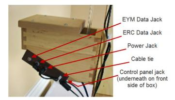
The Ethernet cable runs from the Electronic Control Box to the <u>Control Panel</u>. The Control Panel is your interface with the system. It is a wooden housing with a membrane switch panel that electrically connects to the Electronic Control Box. With the Control Panel you control the following functions:
