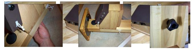
You will then lift the motor housing and insert it onto the HDSS that is lying on the floor so that the bolt of the Nut Plate extends through the hole in the I-beam and faces downward. Attach the knob <u>and both</u> <u>white washers</u> to the end of the bolt while they are in this position. Tighten the knob.
